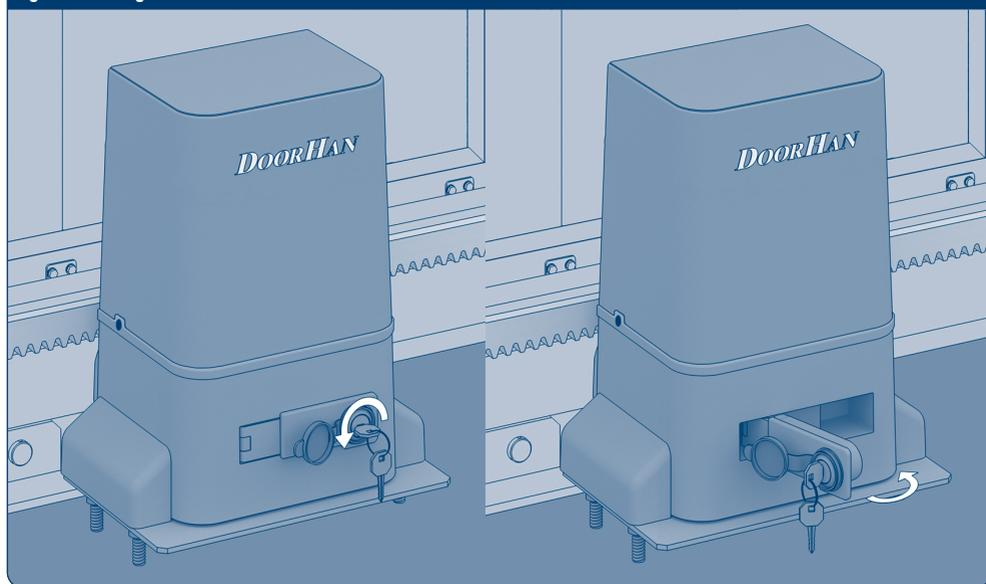
To switch the operator to automatic operation, return the release lever to its original position, turn the key 90° clockwise, pull it out and close the keyhole with a rubber plug (Fig. 2).
